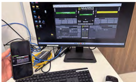
Madrix software powers the screen content, which can also be controlled via AnyDesk from any smartphone
